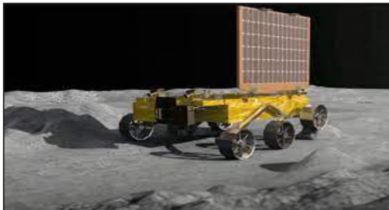
Pragyan rover is a robotic vehicle weighing 26 kilograms, equipped with various instruments.
