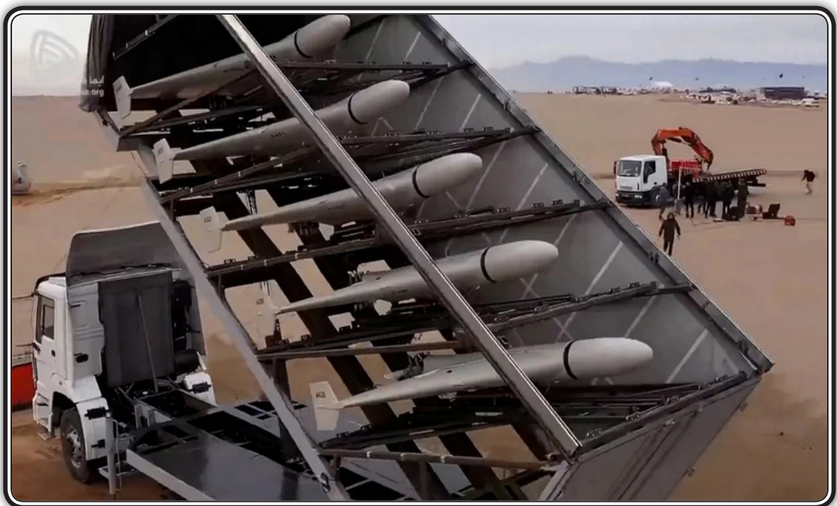
Iran Shahed-136 drones stacked on a launcher before an exercise by the Iranian Army.
