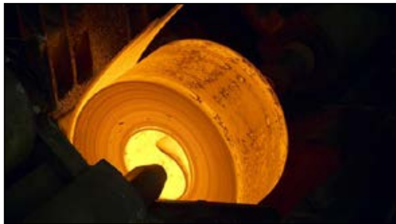
Hot rolled in the form of coil and plate is a type of steel product produced from hot rolling process.
