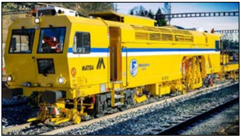
A Matisa plain line ballast tamping machine. Iran's RAI railway company has signed an MoU with Matisa for overhaul and retrofitting of railway maintenance machines.
